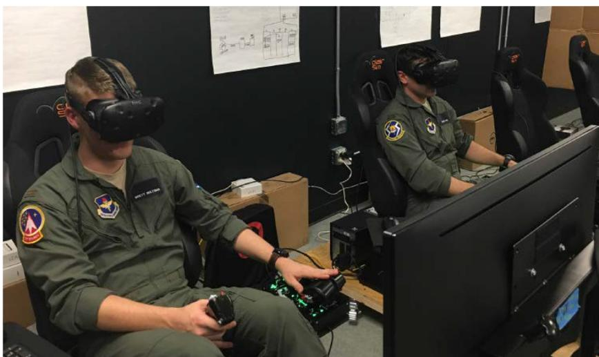
**Figure B-2: Pilot Training Virtual Reality Configuration with Low-Cost Interfacing.**
