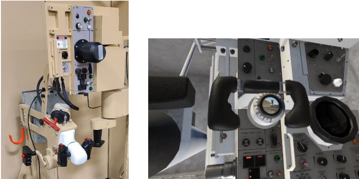
Figure 4. MRTT Physical Hardware Shown on the Left with Trainee VR HMD Display Shown on the Right
