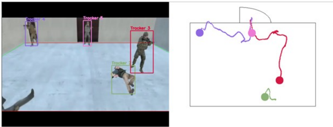
Figure 8: Example of the planar projection from the camera frame (left) to the generated top-down map frame (right).
