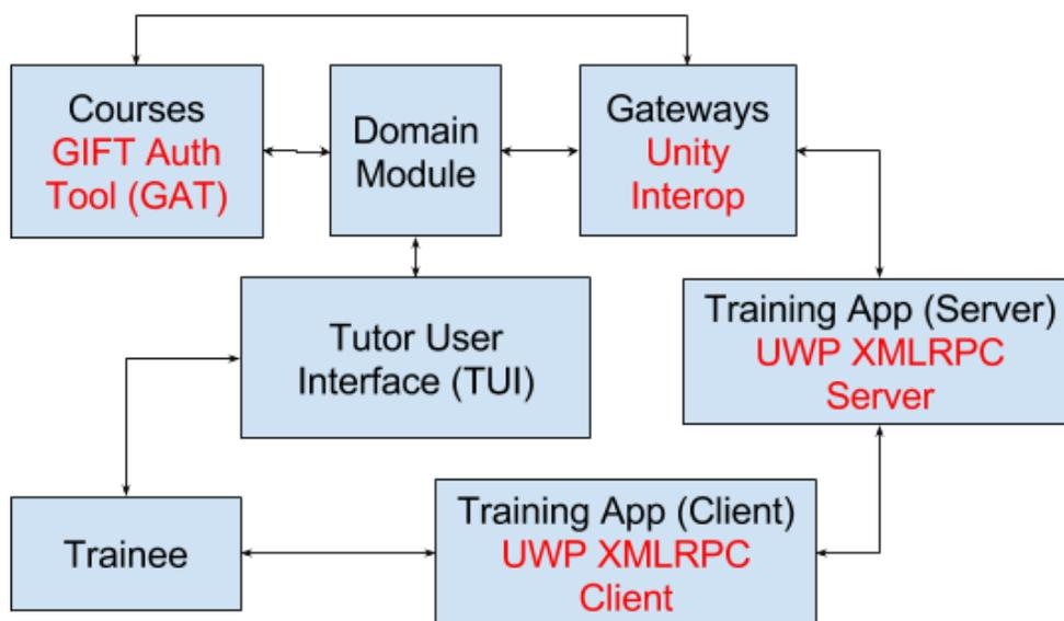
**Figure 2. Modifications made to the GIFT functional blocks. Red text denotes additions to expand functionality. Note the new Unity interop option added in the GIFT Authoring Tool as well as an XMLRPC implementation for Universal Windows Platform.**
